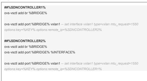
We are connecting the meta channel trough wireguard server and client to form an VXLAN tunnel between our locations.
